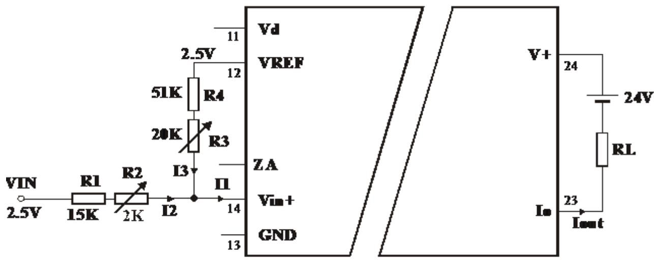
$$I_{out} = \Pi * 100 \quad I_3 = 4mA \quad I_2 = VIN / (R1 + R2)$$
